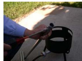
3. *(Long-legged version only; skip this step for the short-legged version)* Slide an adaptor (already on an aluminum tube) into each short leg of the stove, and tighten the other screw on the adaptor so that the stove is upright and stable.
