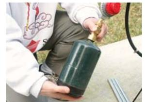
14. **(Steps 12 through 21 are for home stove setup which connects to a regular 20 lbs propane tank.)** First of all, before connecting to the propane tank, detach the bottle adaptor from the hex fitting. Turn the adaptor against the hex fitting clockwise.
