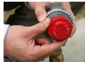
6. Bring together the bottle adaptor end of the regulator from the stove to the propane bottle. Make sure that the adaptor can reach the bottle.
