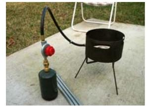
9. Open the regulator valve (turn clockwise as viewed from above) -- slowly. You should now hear a low "hissing" sound (gas flowing out) from the stove's burner outlet.
