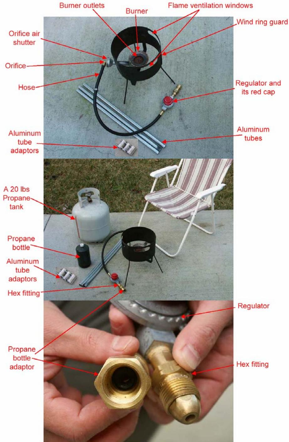
1. Unpack your stove. The stove should come with a wind ring guard, a burner mounted on the wind guard, and a hose with its orifice end already screwed into the burner. On the other end of the hose is a propane regulator with an adjustable red cap and a hex fitting with a propane bottle adaptor which will screw into a propane bottle (not included). If you have purchased the long-legged version, the package will include three (3) aluminum tubes and their adaptors.
