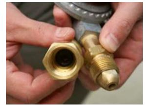
16. With the red regulator tightly in its close (OFF) position, screw the fitting counter-clockwise to the propane tank's connector.
