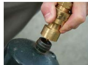
7. Slowly screw the bottle counter-clockwise into the adaptor. The propane gas should start to fill the adaptor up to the regulator. Your hand holding the adaptor should feel cool (by expansion of the gas inside).
