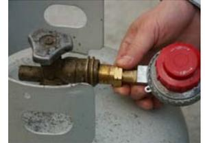
17. **Important!** Before open the propane valve, turn the red cap regulator counter-clockwise fully to shut off the regulator. Open the propane valve (turn counter-clockwise as viewed from above) – slowly, for about one turn (360 degrees).
