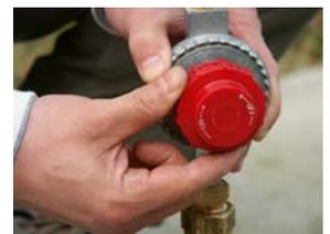
13. Unscrew the propane bottle from the adaptor while holding the adaptor (to prevent accidentally turning the adaptor away from the hex fitting from the regulator).
