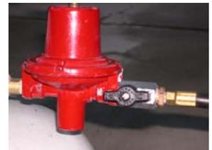
19. Open the regulator valve (turn clockwise as viewed from above) -- slowly. You should now hear a low "hissing" sound (gas flowing out) from the stove's burner outlet.
