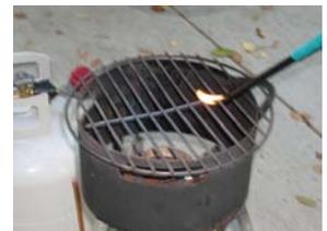
22. Once the flame is lit, adjust the intensity using the (red) **regulator** cap. The more ON (clockwise), the higher power output of the stove. Do not use the propane tank's valve for controlling the intensity of the flame.
