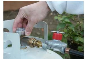
**Caution!** If you hear hissing sound during this step, it indicates there is a gas leak. Return the propane tank valve to its OFF position and make sure the hex fitting is tightly connected to the tank and the regulator is in its OFF position.
