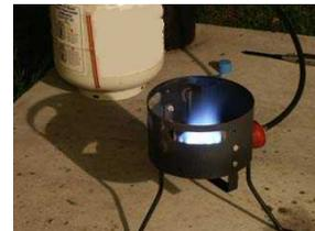
24. Note: If your stove flame is not blue (for example mixed with yellowish flame) or stove low power setting flame is not stable (dies out), adjust the orifice air shutter (refer to the terminology picture on page 1) for a better fuel/air mixture.
