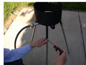
4. Clear the area free of anything that can easily burn or obstruct your cooking. Set the propane gas tank/bottle at least two feet (or 0.7m) away from the stove. The propane tank/bottle (any size, including the camping size) and lighter can be purchased separately from hardware stores, gas stations, or grocery stores.
