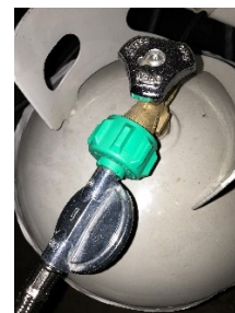
ACME Type I QCC connector clockwise tighten to tank
