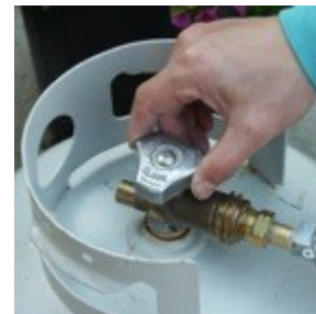
ACME Type I QCC connector clockwise tighten to tank
