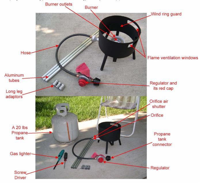
1. Unpack your stove. The stove should come with a wind ring guard, a burner mounted on the wind guard, and a hose with its orifice end already screwed into the burner. On the other end of the hose is a propane regulator with an adjustable red cap and a hex fitting that will screw into a regular propane tank (not included). If you have purchased the long-legged version, the package will include three (3) aluminum tubes and their adaptors.
